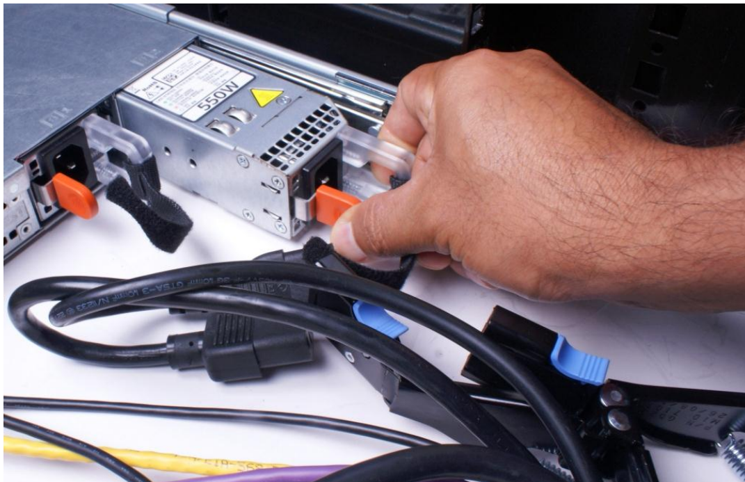
Figure 9. Replacing the outer power supply
