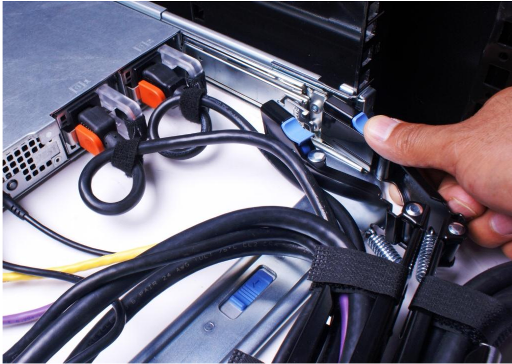
Figure 8. Disconnecting the CMA attachment housings
