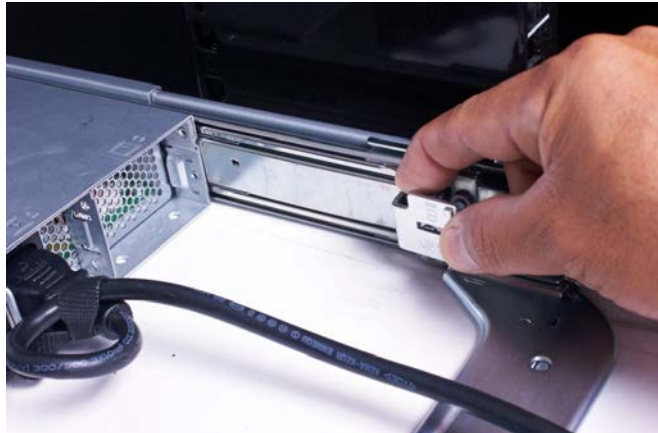
Figure 4. Attaching the inner CMA attachment bracket
